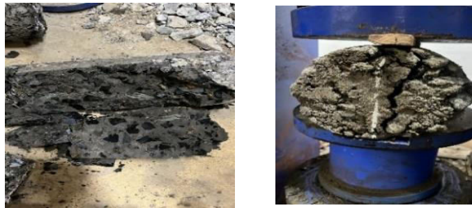
Fig. 8: Split tensile strength testing on Tensile strength of concrete
